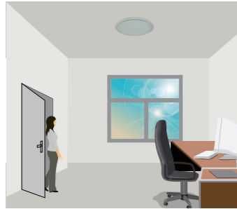
With sufficient natural light, the light does not switch on when presence detected.
