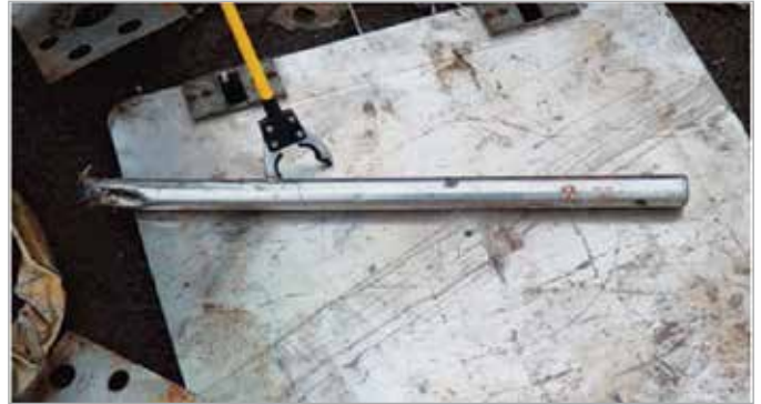
50 mCi AmBe industrial source found in steel scrap
