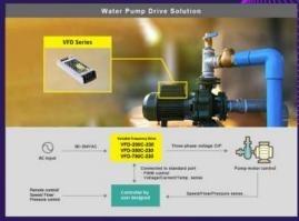
These controllers are suitable for use in applications such as smoke extraction equipment and water pumps.
